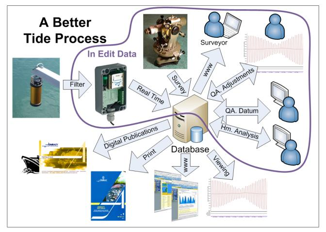
Here we've outlined the work in progress with a purple line on the diagram. This is the data that is being worked on by the hydrographer. It takes time. She doesn't want to publish it until the work is finished. Traditionally, keeping this data separate involves manually taking a copy of the files to work on. This is tedious and error prone. Tedium is what computers are best at. It is simple for a computer program to do this and to always do it accurately.
