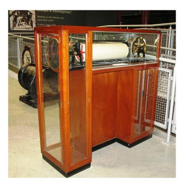
Drum tide recorders are well known and quite simple, obvious devices. They record 14 days of tide on a single drum that rotates once every 24 hours. Brunel knocked this one up in a spare moment from building bridges, tunnels, railway lines, and the odd ship or two.
