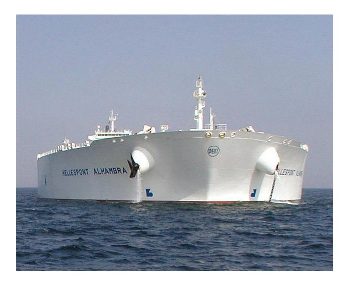
When can a supertanker like this transit the Malacca Strait? The strait is only 23m deep at its shallowest. The navigator has to time it just right to have enough water under the keel.
