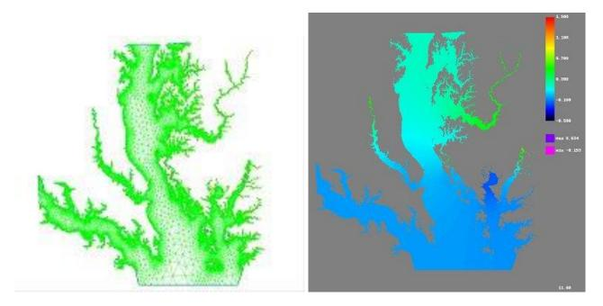
NOAA have developed a system called TCARI which provides continuous tide height from just tide gauge data. It works by interpolating each component of the water height separately using a mesh. A separate analysis is done for the vertical datum, each harmonic component and the residual.
