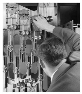
On the right, you can see how the mechanism converts rotation into a sine function using a pin in a slot.
