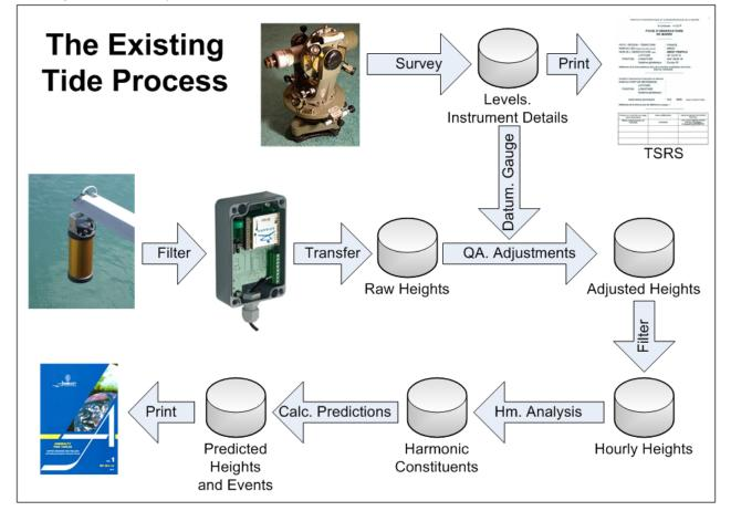
Here, again, is the computer based process that is common now. This is very similar to the earlier process, but with computers instead of mechanical machines to do the calculations, and computer files instead of paper to store the results.
