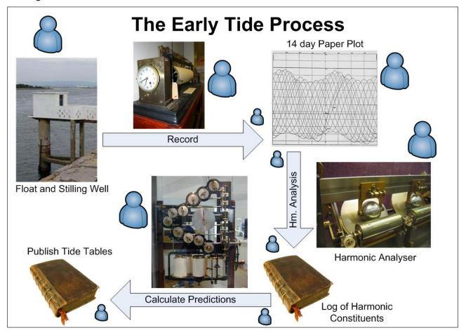
Here we can see the skilled steps in the process, which I've shown with the larger blue people. Just keeping these mechanical wonders working was skilled. Keeping the float and wires working freely. Changing the paper on the drum recorder whilst ensuring that its clock is correct. Transcribing the data from the drum paper. Checking the data. Choosing the harmonics for the analysis.
