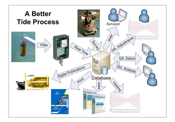
So we put a database at the centre of operations. There are still skilled tasks for people to perform such as checking and analysis, but the database is used do the mechanical simple things like retrieving the correct data for a particular station.
