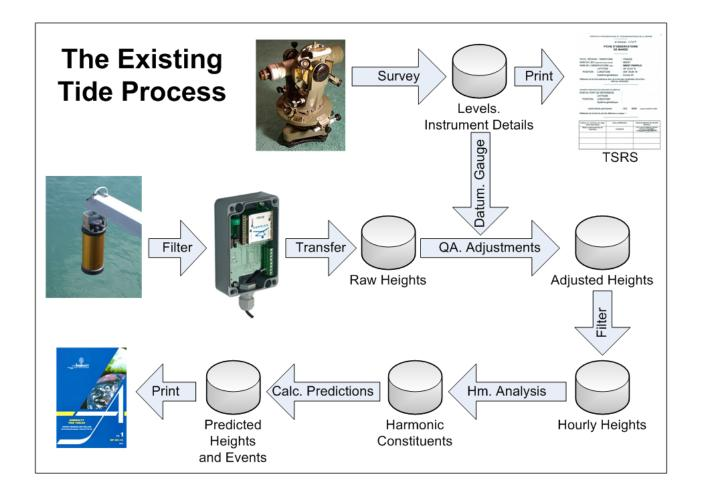
The computer disk is like a large filing cabinet. There are lots of steps in the tide process. Separate files are used to store the results of each step. These are the drums in this diagram.
