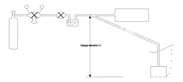
The first successful one was the bubbler pressure gauge (pictured above) which is based on Archimedes principle.
