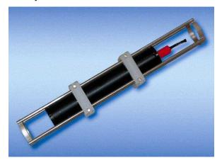
Later still, we have some modern gauges. On the left is a direct pressure sensor gauge made by Valeport. This is particularly useful offshore – one can be simply dropped over the side and left on the sea bed for a month or two happily recording away. The gauge is then recovered and its data extracted.
