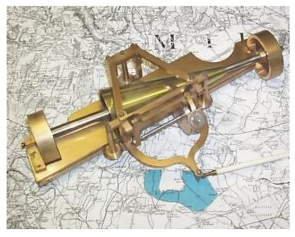
The basic process of mechanical integration already existed in a machine called a Planimeter which calculates, for example, the area of a field on a map. Its central component is a continuously variable gear – that is the cone in the picture. The output is the area within the curve followed by the stylus. Thomson's genius was that he realised he could do a similar thing with a tide height graph as input. The output would be the harmonic constants.
